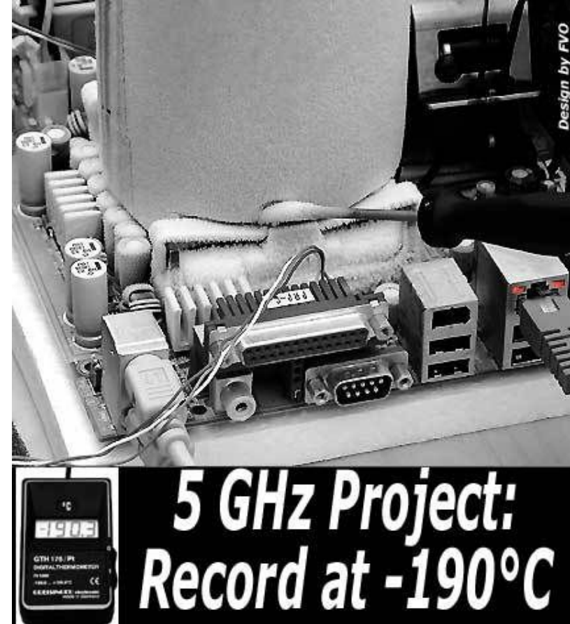
Nitrogen-cooled Pentium 4 (5.25 GHz, 2003)
