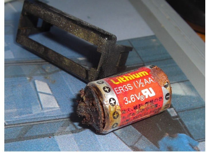
Leaked ER3S battery
